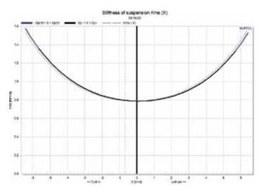
Figure 12b: Stiffnes of suspension after optimization.
