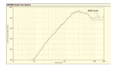
Figure 7: Effect of acoustic lens.
