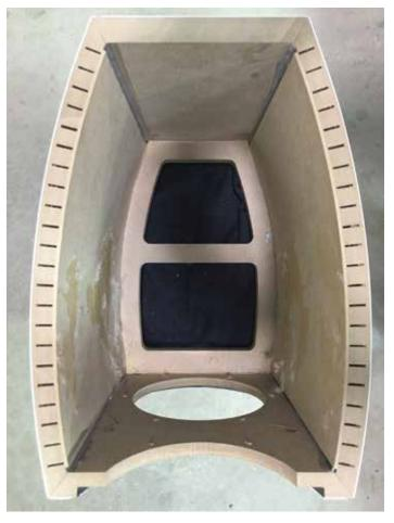
Figure 13: Cross section of Concerta2 F36 baffle showing the Kerf technique.
