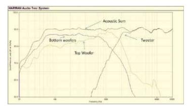
Figure 2: Acoustic Response of each driver, F35.
