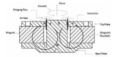
Figure 10: Electromagnetic principal.
