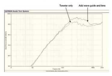
Figure 6: The gain advantage of the Concerta2 tweeter over no wave guide.
