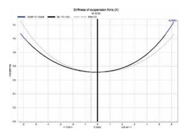
Figure 12a: Stiffness of suspension before optimization.
