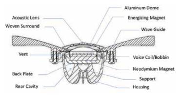
Figure 4: Cross sectional view of the Concerta2 tweeter/waveguide assembly.
