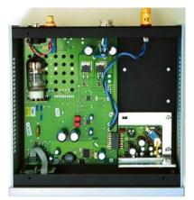
Pro-Ject puts an ECC88 tube in the prepuffer-stage. After that the signalpath continues stricly digital. The PSU is completely external.
